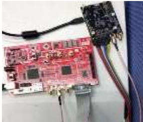
Clock Glitch Against Glitch Detector Structure in 12 th Generation Intel Core Processor [5]
